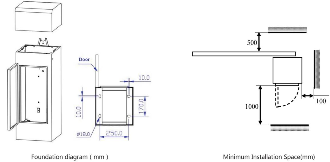
1. Fix those 4PCS expansion bolt (M16\*120) on the concrete foundation according to above Foundation Diagram in "4.3 Foundation" ;
