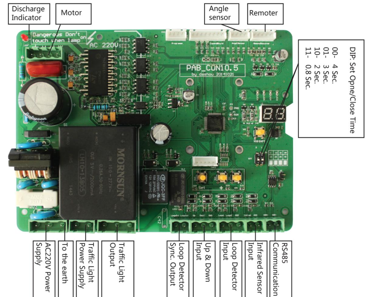
Caution 1: While Discharge Indicator working, Don't touch the left side part of the board. The board is divided into left side part and right side part by a middle white line. The process of Discharge last about 5 minutes.
